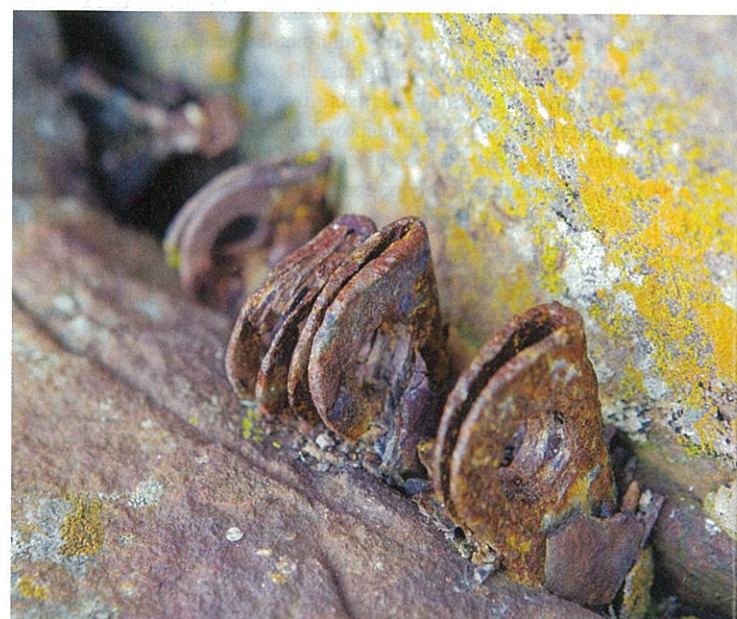
From the sea stacks of Scotland (images one, two, and four) to the beaches of the Dominican Republic (image three), saltwater accelerates the rusting of all types of metals, including aluminum and various kinds of steel.
